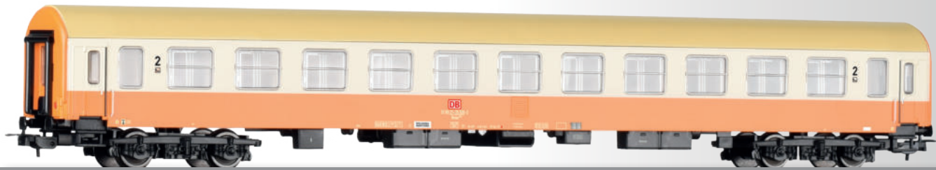
Reisezugwagen 2. Klasse Bomz 283, Bauart Halberstadt, der DB AG 2nd class passenger coach Bomz 283, type Halberstadt, of the DB AG
