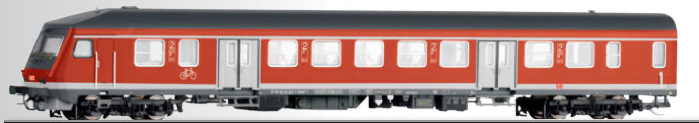
Steuerwagen 2. Klasse Bybdzf 482 der DB AG 2nd class driving cab coach Bybdzf 482 of the DB AG
