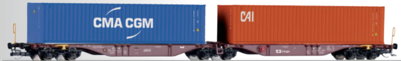
Containertragwagen Sggmrss 578.0 der ČD Cargo Container car Sggmrss 578.0 of the ČD Cargo
