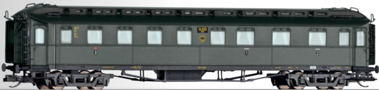
Reisezugwagen 1./2./3. Klasse ABC4ü der DRG 1st/2nd/3rd class passenger coach ABC4ü of the DRG
